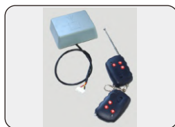
Remoter: transmitter, distance>20m
